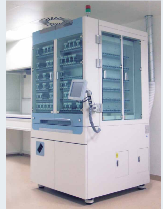
GMP clean room with automatic blister packaging machine and deblistering workplace
