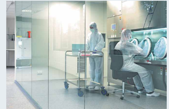
Individual clean room equipment with cytostatic safety cabinet, insulator technology and material airlocks
