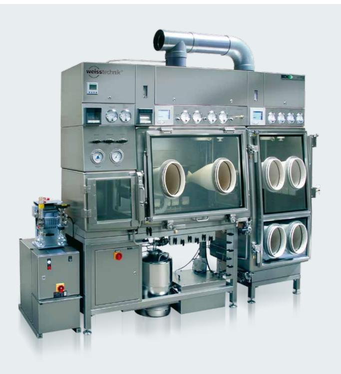
Insulators can be used anywhere where a controlled atmosphere needs to be created away from the installation room. In addition, they offer optimal protection for products and employees. Depending on the area of application, insulators are operated at underpressure for protection of persons and the surrounding area and at overpressure when solely providing product protection.
